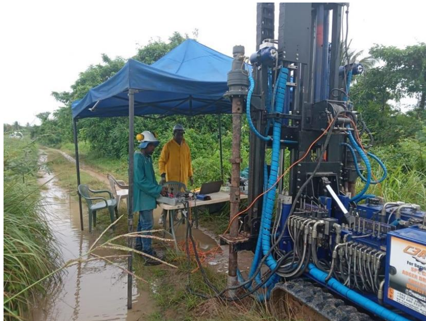
Figure 2: CPT operation at Leguan, Region No. 3
