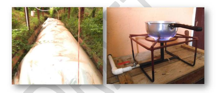
GEA, with support from UNDP and OPM, installed an additional two bio-digesters in 2012. In an effort to promote the use of bio-digesters in farming communities, GEA has prepared a "Guide for the Design and Construction of Low-cost Bio-digesters" which can be used by small scale farmers to convert animal waste to energy in the form of biogas which can be used for cooking, lighting and electricity generation.
