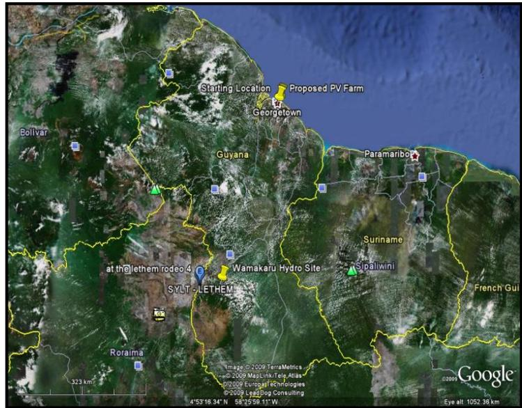
The Wamakaru site is located between 790 and 1575 feet near the north-eastern end of the Kanuku mountains, some 40 km (25 miles) north-east of Lethem and 17 km (10 miles) south-east of the village of Nappi. A power house of two 250 kW and three 750 kW generating units (total 2,750 kW) was initially contemplated.
