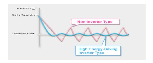
Air conditioners convert a large amount of thermal energy and therefore have high power consumption...
