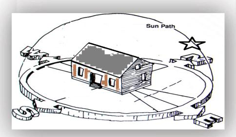
Buildings should be oriented in the east to west direction to minimize the effects of the sun and to maximize the wind draft.
