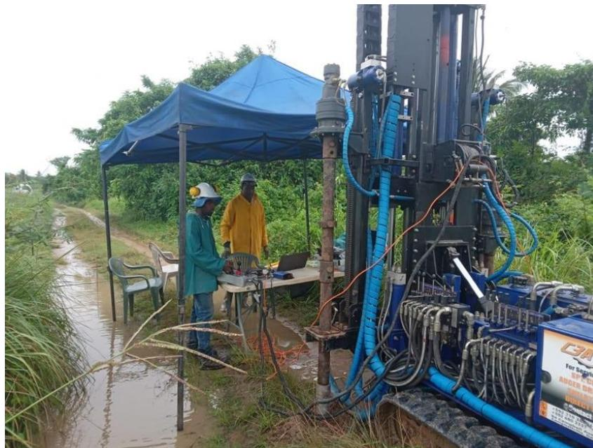
**Figure 2: CPT operation at Leguan, Region No. 3**
