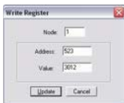
Fig. 269: Write register - acknowledge alarm message
