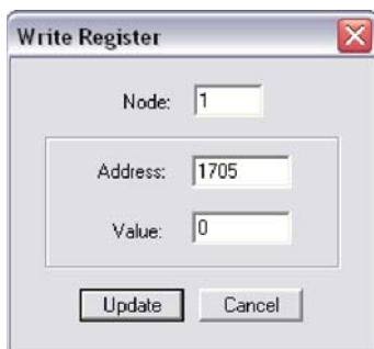
Fig. 273: Write register - enable the resetting procedure via RS-232/RS-485
