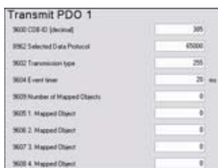
Fig. 181: TPDO configuration for IKD 1 (example Toolkit)
