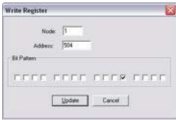
Fig. 234: Modbus - write register - external acknowledge
