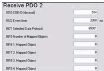
Fig. 191: RPDO configuration for 2nd IKD 1 (example ToolKit)
