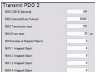
Fig. 189: TPDO configuration for 2nd IKD 1 (example ToolKit)
