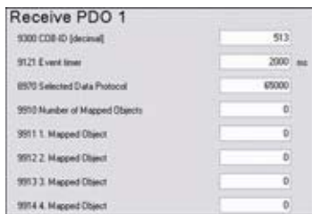
Fig. 183: RPDO configuration for IKD 1 (example ToolKit)
