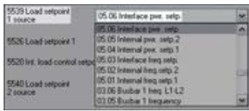
Fig. 238: Setpoint source configuration
